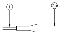
Style 34 1: 75 cm capillary 2: 1/4" tube for braze connection
